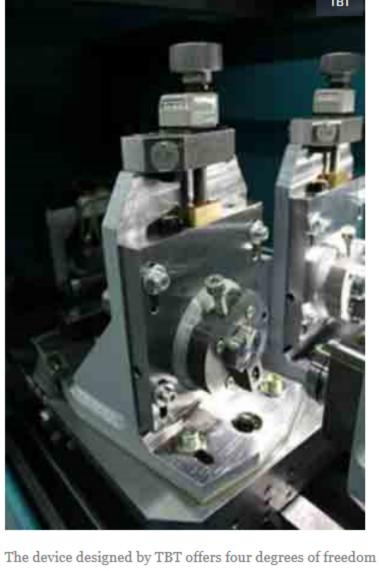
for workpiece adjustment. The photo shows the scale for the 360° rotation of the workpiece and the counter for height
