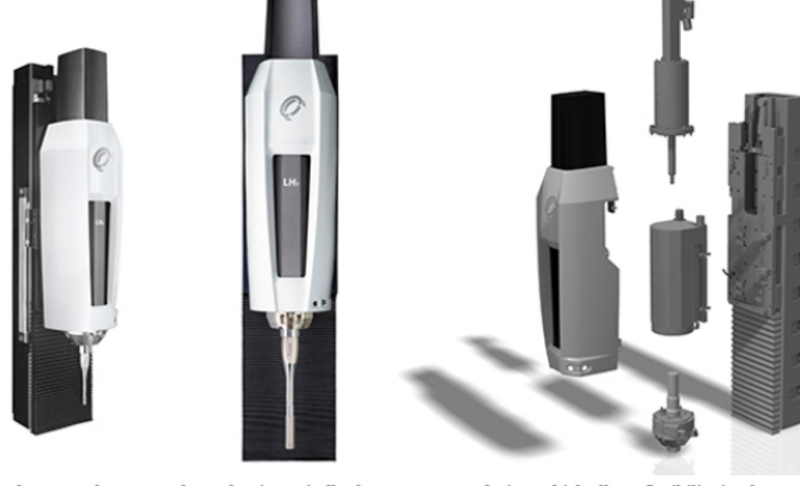
Left and center: The LH2 and LH3 honing spindles have a compact design, which allows flexibility in placement and keeps energy requirements low. Right: The LH spindle and expansion motor are arranged coaxially, one above the other. There is no bending or tilting torque caused by lateral drive components.
