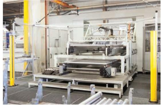
which the tool is expected to achieve, can be set via two different workpiece counters, which trigger different reactions in the program execution. This means the machine stops for a change of cutter in good time before tool failure. The ML500 also has feed force and coolant pressure monitoring. If the wear and tear on a tool should exceed a certain level more quickly, or if any other problem arises, the machine will also shut down automatically.
