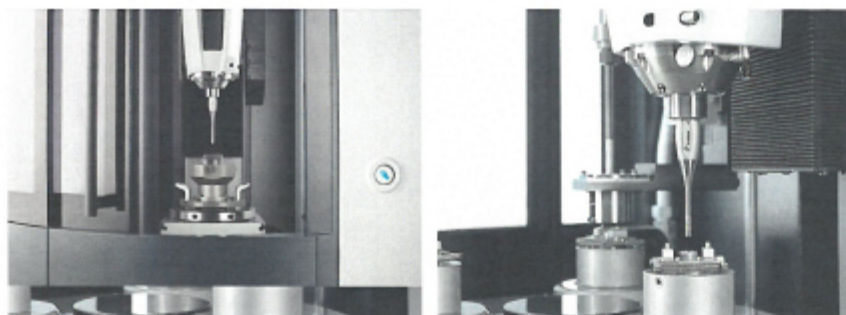
The E line can be equipped with a fixed table (left) or a rotary table with up to three workstations
