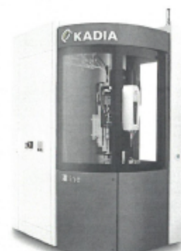
The E line is a compact honing machine that takes up just 2.5m 2 of space
