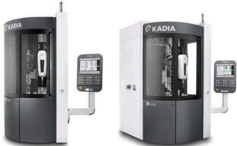
The E line is a compact honing machine that takes up just 2.5 m 2 of space
