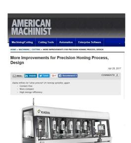
Every micrometer counts when it comes to honing of high-precision components, such as those required for injection or hydraulic applications. To meet those high quality standards, honing machine manufacturer Kadia Produktion GmbH + Co. applies directdrive technology for the spindles and the stroke. Meanwhile, it has introduced the second generation of its LH honing spindles.
