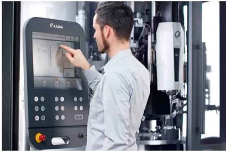
With the HMC100 machine controller, the operator gets the most out of his LH honing spindles.
