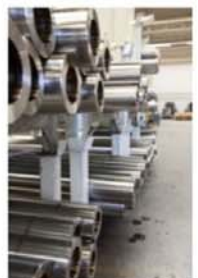
Components at GLUMANN Maschinenbau, which were drilled on the ML500 deep hole drilling machine from TBT
