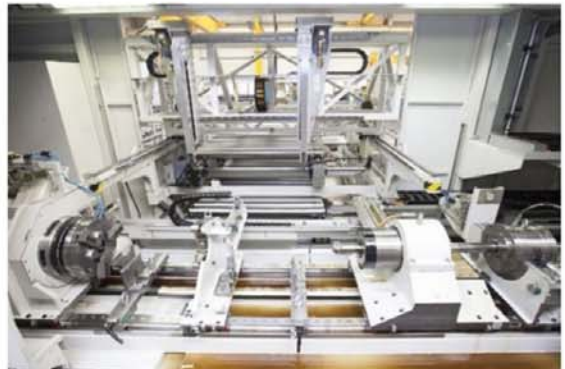
The loading and unloading unit behind the machine provides good access, making it easy to bring in and remove the components
