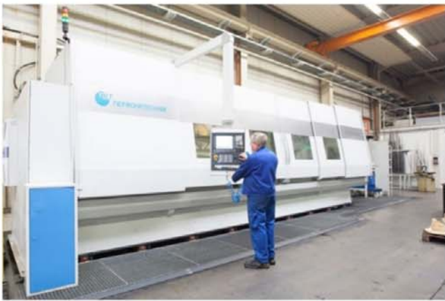
Deep hole drilling machine type ML500 from TBT at GLUMANN Maschinenbau in Chemnitz. The machine is used for drilling holes with diameter up to 80 mm and depth up to 2000 mm using BTA/STS technology.
