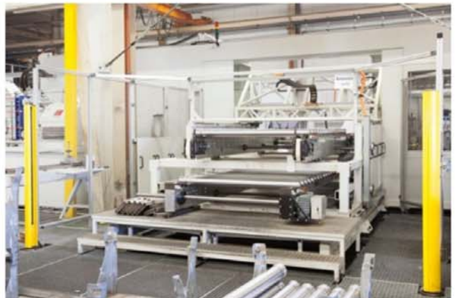
The components are loaded onto conveyor chains, on the upper level are the components to be drilled, and on the lower level are the components which have been drilled. On the left is the adjustment spindle for setting component length.
