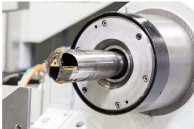
GLUMANN drill using the BTA/STS process on the ML500. Cuttings and cooling lubricant are fed out of the working piece through openings in the drill head
